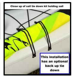
Another thing to consider, before installing a tie down kit, is to see if your boat already has lines or bungee cords that will be helpful in securing the sail when it is down. Many times boats will have existing shock cords that are convenient for securing the sail. If you plan on using a shock cord that is already on your boat, make sure it will hold the sail securely so it stays in place as necessary.
