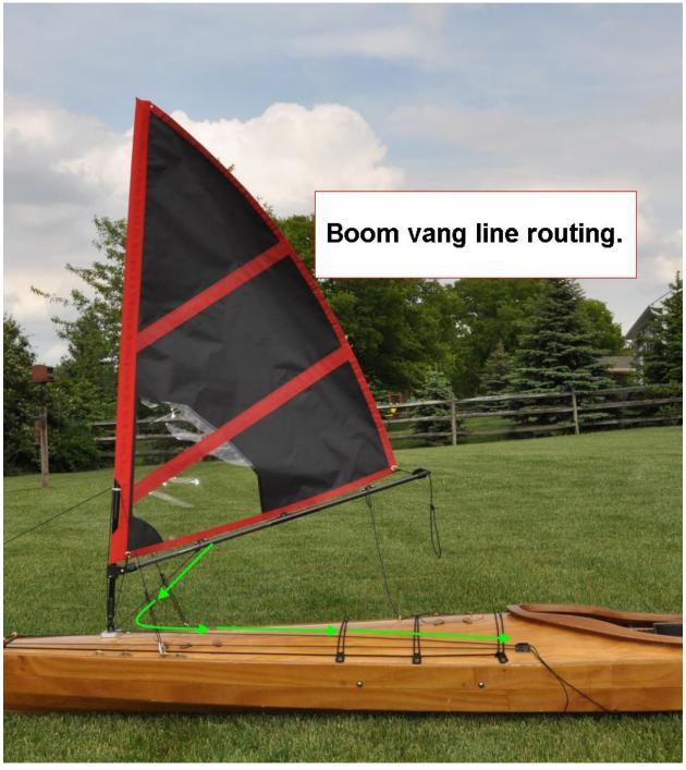
This picture shows an overview of the routing of the boom vang line.
